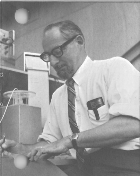
In a cryogenic temperature experiment with liquid nitrogen, Al Benjaminson, manager of transducer engineering, uses a new quartz thermometer (on shelf above) for ultra-precise measurement.
